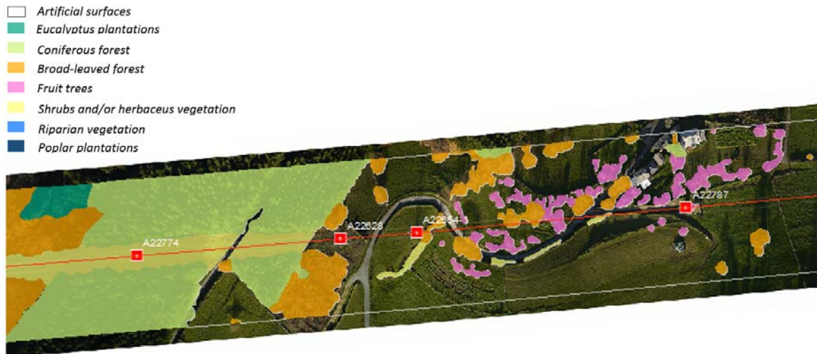
Figure 2.2. Result of the identification of the type of vegetation in a section of line.
